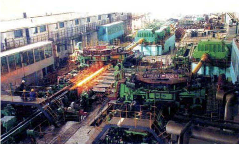
The \phi 180mm Accu-Roll Precision Hot Pipe rolling Plant.
